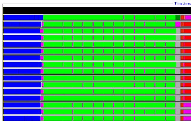
Fig. 6. Example: Taylor order 12, System order 32, 16 procs., computation time \sim 2 min. - Time shares: Fixed Point Iterations (Blue) - LS Computation (Green) - LSS (Red) - Comm.+Idle (Magenta)
