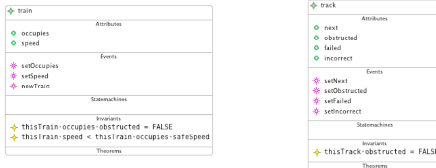
Fig. 7. The refined model consists of the two refined classes with all their previous attributes and associations inherited (i.e. retained) and some new invariants added.
