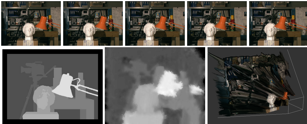
■ Figure 4 The extended Tsukuba dataset from the Middlebury stereo benchmark [10]. The five source images, reference depth map, our resulting depth map, and a 3D rendering of the result.
