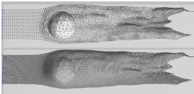
■ Figure 14 Triangulations of an adaptive (top) and a high-resolution non-adaptive streak surface passing a spherical obstacle. Triangle counts in the time step shown evaluate to approximately 20.000 and 45.000. The adaptive surface yields a highly diverse particle density, while accurately representing fold-like features.
