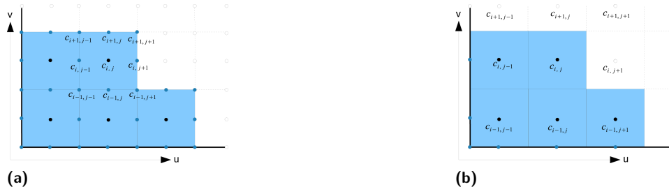
■ Figure 1 (a) Initial distribution of the basis coefficients defining corresponding biquadratic B-spline functions within an adaptive quad-grid consisting of empty and non-empty quadrilateral. Blue points represent zero-valued basis coefficients located at the domain boundaries of the data set having knot multiplicity three, black and white points are basis coefficients having knot multiplicity one. The white points are zero-valued basis coefficients of empty quadrilaterals. (b) quad-grid after knot removal.
