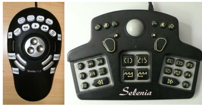
■ Figure 7 Left: A general function pad may be used to provide fast access for the most important interactions. Right: A dedicated function pad has been developed and refined in various iterations to provide fast access to frequent commands in a diagnostic system for mammography data. (Right image: Courtesy of MeVisBreastCare)
