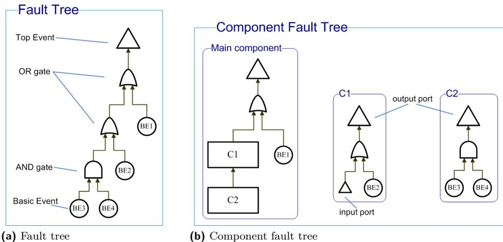
■ **Figure 1** Fault tree and component fault tree. (a) A fault tree consisting of four basic events connected by an AND-gate and two OR-gates. (b) The component fault tree model based on the fault tree in (a), which contains a main component and sub component “C1” and “C2”. “C2” inputs its failure to “C1” via ports.
