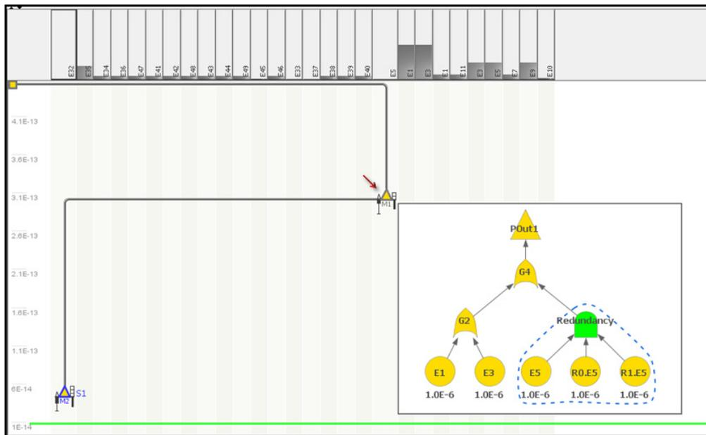
■ **Figure 6** Pop-up window shows the updated logical structure of the CFT component with respect to the modification “M1”. The new created sub-tree is arranged in a scope having a dotted border. Two basic events were added and connected with the initial basic event using an AND-gate.
