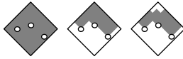
Figure 1: Trimmed evaluation. Originally, Yates’s algorithm considers the entire subset lattice (left). We trim the evaluation from below by considering only the supersets of ‘interesting’ points (middle), and from above by abandoning computation when we reach certain points (right).
