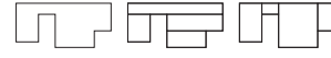
■ Figure 3 A shape to be formed (left) and the possible rectangle decompositions thereof (middle, right).
