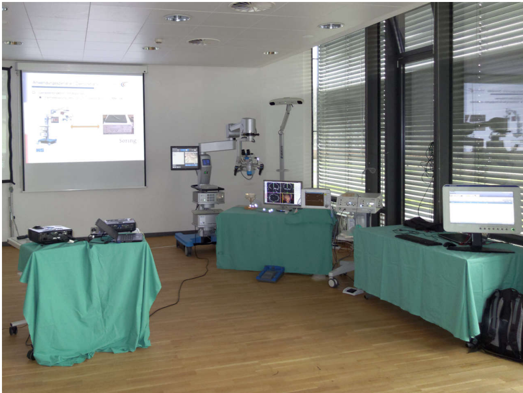
■ Figure 7 Image of an openSDC powered distributed system of medical devices at a project workshop in December 2013. F.l.t.r.: operating microscope, navigation system, patient monitor, ultrasound surgery device and documentation system.
