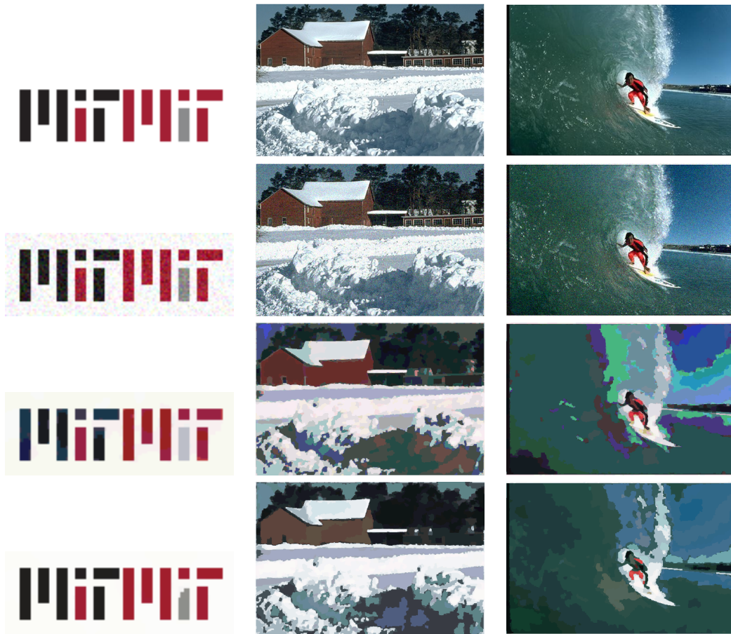
■ Figure 1 MIT logo (first column, size 45 * 124 ), and two images from the Berkeley segmentation dataset [26] (second & third columns, size 321 * 481 ). The first row shows the original image; the second row shows the noisy image; the third row shows the denoised image using full color space; the fourth row shows the denoised image using image space (our algorithm).
