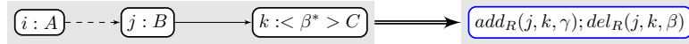
■ Figure 5 An example of LDRS. The dashed line represents the program (label) \alpha and the plain line the program \beta . The first edge labeled \beta after an access \alpha on a path toward a C gets a new tag \gamma .
