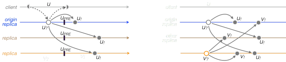
(a) Operation u decomposed into indivisible call, return, generator u_? and effector u_! . Precondition u_{PRE} is true at the effector. (b) The effectors of concurrent operations may execute in different orders in the general case.
