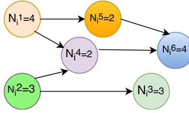
■ **Figure 1** A DAG  $\tau_i$  with total execution time  $C_i = 18$  and minimum inter-arrival separation  $T_i = 12$ . It is a heavy task since  $C_i > T_i$ . The path  $\mathcal{N}_i^1 \rightarrow \mathcal{N}_i^4 \rightarrow \mathcal{N}_i^6$  is the critical path with minimum makespan of  $P_i = 10 \leq T_i$ . As a result, this task may meet its deadline provided enough processors.
