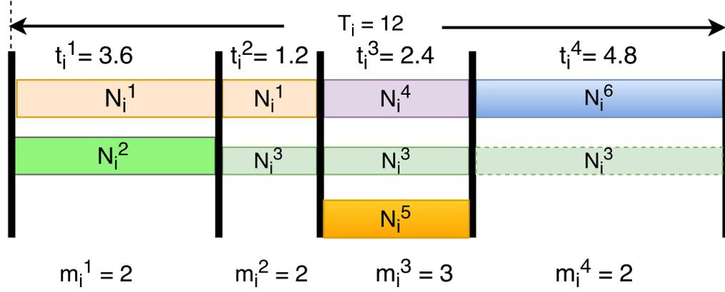
■ **Figure 4** The segment-node mapping for  $\tau_i$  (in Figure 1) after segment extension. Scheduling windows for the nodes become  $[1, 2]$ ,  $[1, 1]$ ,  $[2, 4]$ ,  $[3, 3]$ ,  $[3, 3]$ ,  $[4, 4]$  respectively, which results in an average power consumption of 3.08 Watts. The height of each block represents the speed of the processor during each segment.
