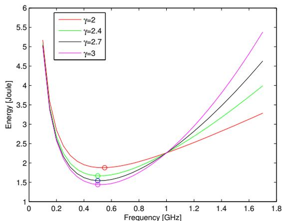
■ **Figure 2** Energy consumption for executing a job with  $10^9$  computation cycles under various  $\gamma$  values, where  $\alpha = 1.76 \text{ Watts}/\text{GHz}^\gamma$  and  $\beta = 0.5 \text{ Watts}$ .
