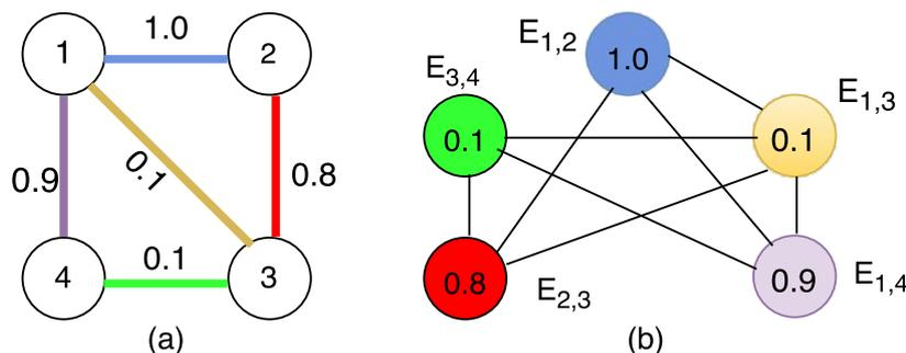
■ **Figure 7** The equivalence of the MPS problem and the MIS problem, where (a) shows a DAG of four processor assignments with potential power savings for merging each pair of the processors, and (b) shows its alternative (equivalent) expression with vertices representing all edges in (a), and edges representing the mutual exclusive constraints.
