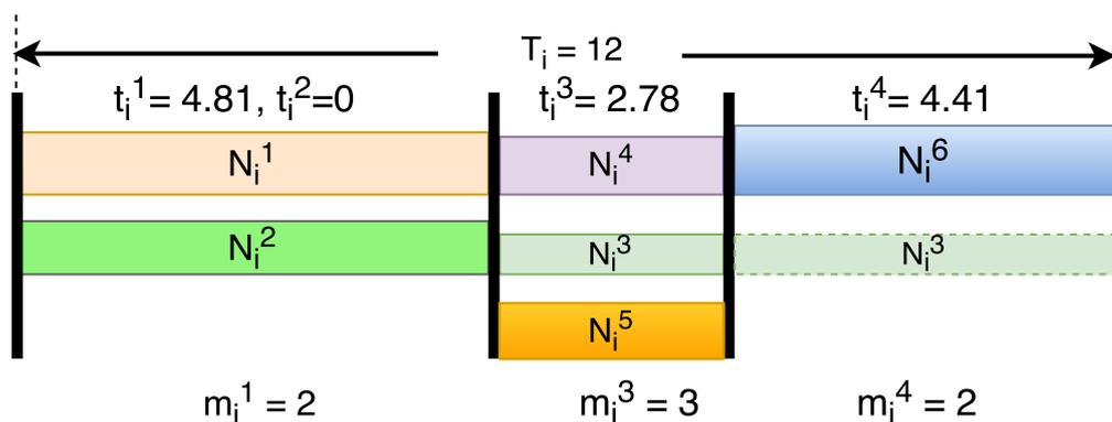
■ **Figure 5** The sub-optimal segment length assignment for power efficiency of the sample task  $\tau_i$  (in Figure 1), with an average power consumption of 2.94 Watts. The height of each block represents the speed of the processor during each segment.
