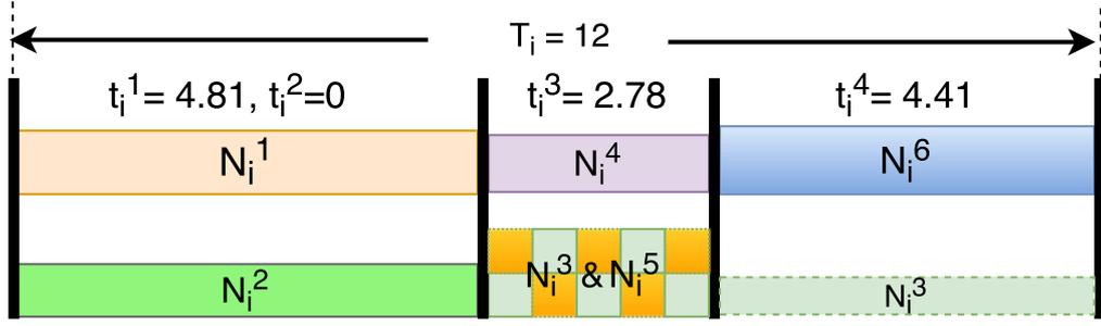
■ **Figure 6** The execution pattern for  $\tau_i$  (in Fig. 1) after merging Processors 2 and 3, where Nodes  $\mathcal{N}_i^3$  and  $\mathcal{N}_i^5$  will share Processor 2 (i.e., execute under EDF) within time window  $[4.81, 7.59]$  at a higher execution speed. The average power consumption is further reduced to 2.80 Watts. The height of each block represents the speed of the processor during each segment.
