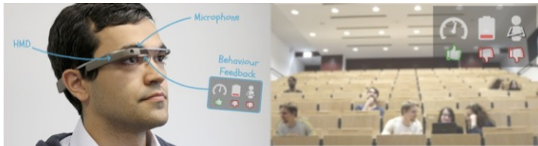
■ Figure 1 A user wearing an HMD while giving a lecture (left). Using various sensors and social signal processing techniques, the user receives real-time feedback on his behavior superimposed on his field of view (right)
