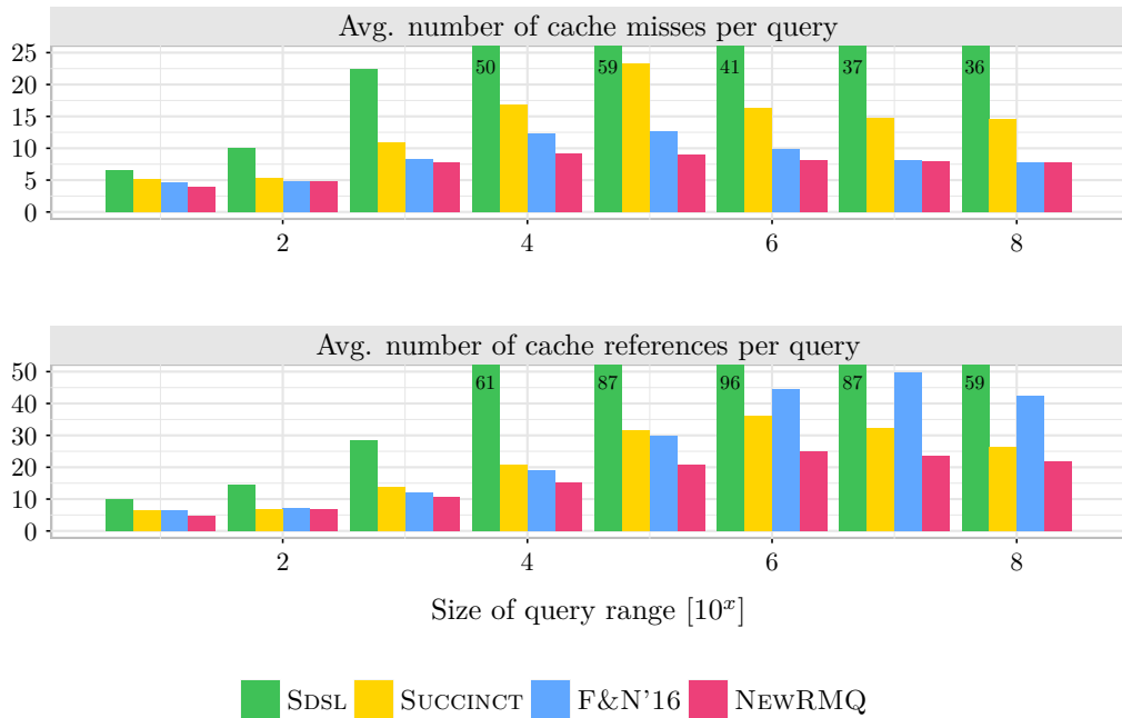
■ Figure 7 Cache access statistics for all implementations on input RANDOM of size n = 10^9 .
