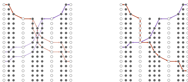
■ Figure 3 Tiny example with two trains running in opposite directions on a single line track with two passing possibilities. The white nodes have capacity 2, the other nodes have capacity 1. Nodes in the same row correspond to a sequence of stations at the same time step, nodes in the same column correspond to one station but at different time steps (time grows from top to bottom). All arcs are single track. The left picture shows an optimal solution for the standard linear relaxation. Note that the solution exploits the weak formulation allowing the two trains to meet and pass on a single line part. The right picture shows the optimal solution if the strong configurations of Section 5.3 are used: one train has to wait at a capacity 2 node for the other train to pass.
