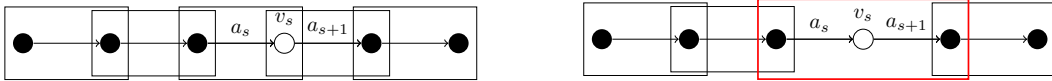
■ Figure 5 The left picture shows the structure of single-arc only subproblems. The right picture shows the case with the new siding configuration, which covers the arcs adjacent to v_s .
