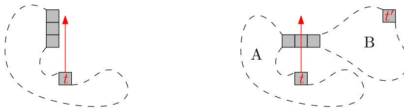
(a) If the removal direction of t is not crossed, the last blocking tile has to be convex (and has to be removed before). (b) If the removal direction of t crosses P , then P gets split into components A and B . Component B has a convex tile t' that needs to be removed before t .
