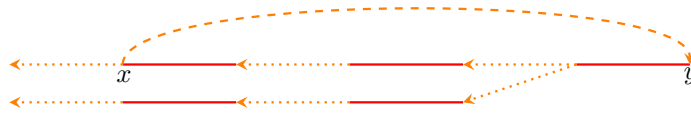
■ Figure 6 Red solid lines represent edges in M . Edge xy is added to a Directed Semi-Matching because there exists a directed path starting from xy and not visiting x . The other orange dotted lines represent edges stored in Directed Semi-Matchings in previous iterations.
