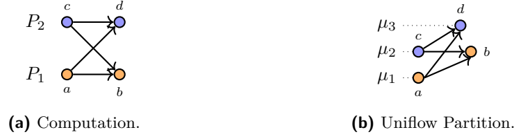
■ Figure 6 A computation on two processes in: (a) its original non-uniflow partition, (b) equivalent uniflow partition.
