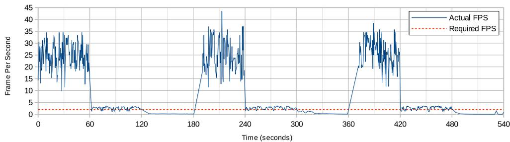
■ **Figure 13** FPS over time – Motion Detector component.
