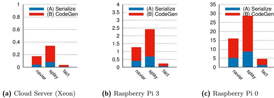
■ **Figure 8** Serialization / Code Generation Time (in seconds). Margins of errors were between 0.5% and 5% for all results, for a confidence interval of 95%.
