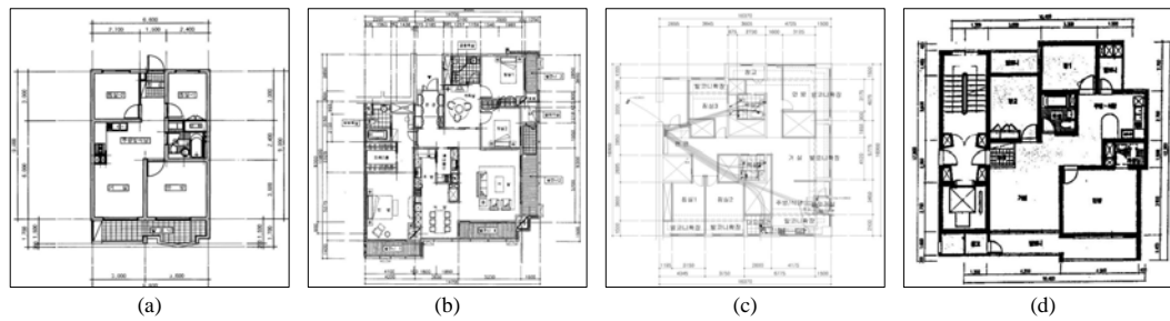
■ Figure 2 Different floorplan formats: (a) format with simplified walls, (b) format with bearing walls, pillars and the interior symbols, (c) format with the electronic wiring, (d) format with different representative of walls.
