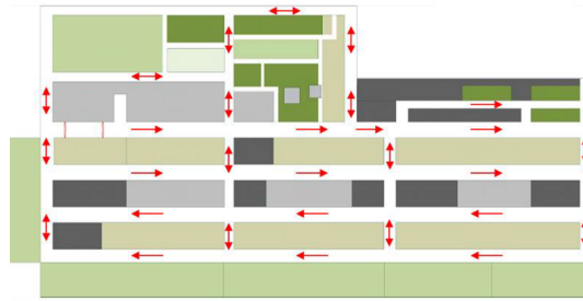
■ Figure 3 Real-world factory layout with transport corridors and directions indicated by arrows.
