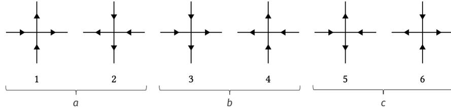
■ **Figure 1** The valid edge orientations for internal vertices in the six-vertex model.
