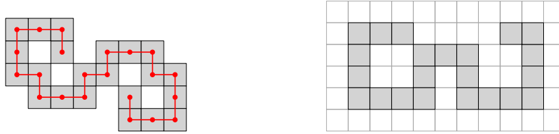
■ Figure 3 Left: a rigid configuration of edge-connected pivoting squares. Right: A configuration that can be reconfigured into a strip, in spite of containing instances of the three forbidden patterns.
