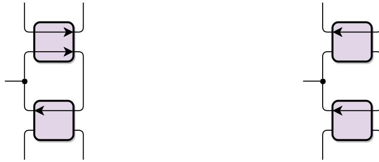
(a) An edge gadget pointed up, in the unlocked state. The gadget is accessed by the loose end on the left.
