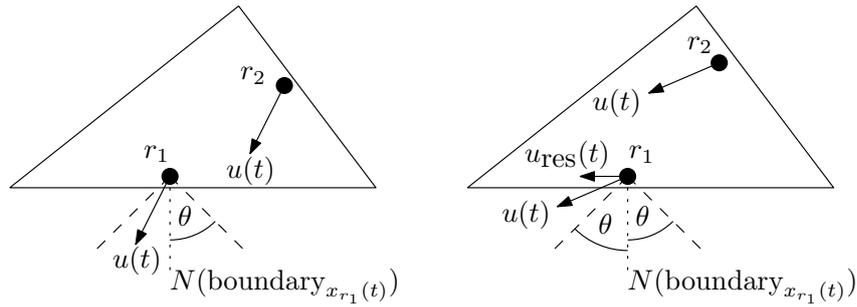
■ **Figure 1** Left: An input force command  $u(t)$  within the cone  $\pm\theta$  about the normal to the boundary results in no motion of  $r_1$ . Right: An input force command  $u(t)$  outside the cone results in a motion of both particles. Observe that  $r_1$  slides along the boundary with a resulting force  $u_{\text{res}}(t)$ .
