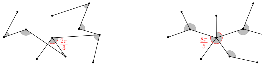
■ Figure 1 Left: A 120^\circ -ST ( \frac{2\pi}{3} -ST). Right: a degree-5 minimum spanning tree which is a \frac{8\pi}{5} -ST.
