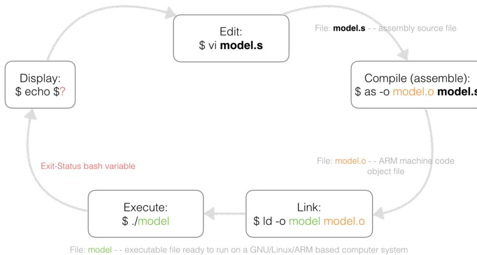
■ **Figure 4** Workflow to test each assembly program into the bash GNU/Linux Operating System.
