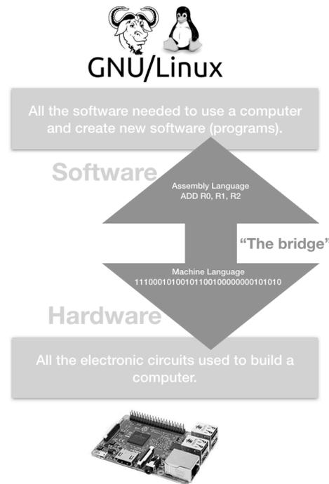
■ **Figure 1** Assembly language, the bridge between hardware and software (adapted from Dunne (2017) [4]).
