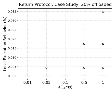
(b) The percentage of local execution behavior for different probabilities of unsuccessful offloading operations under the return protocol and 20% offloaded workload per task.
