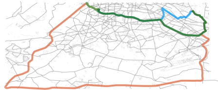
■ Figure 2 Visualization of example routes: original route (blue), optimal alternative routes with respect to the User Equilibrium for SAP (green), for 1D-SAP (black), and D-SAP (orange).
