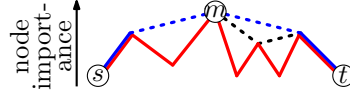
■ Figure 2 Solid lines are edges in G . Dotted lines are shortcuts. Red is shortest st -path in G . Blue is equally long up-down st -path in G^+ . m is the mid node.
