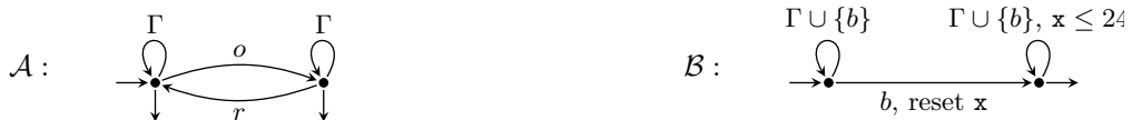
■ Figure 1 Left: a finite automaton \mathcal{A} recognising language \Gamma^*(o\Gamma^*r\Gamma^*)^*(\{\varepsilon\} \cup o\Gamma^*) , where occurrences of o are interleaved by occurrences of r . Right: a timed automaton \mathcal{B} with single clock x .
