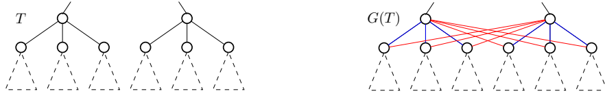
■ Figure 4 Connecting levels of the selector tree. Blue/red edges on the right symbolize true/fake edge gadgets.
