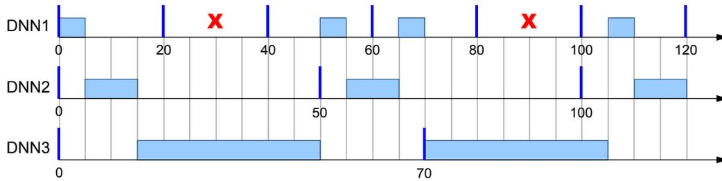
■ **Figure 1** Example of non-preemptive schedule of three DNNs with different execution times and periods. As clear from the figure, DNN1 experiences longer and variable delays.
