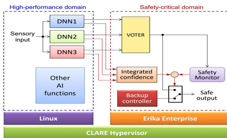
■ **Figure 7** Architecture scheme proposed in [8], including a high-performance domain (running all the AI functions) and a safety-critical domain (running all critical control functions), managed by the CLARE hypervisor.
