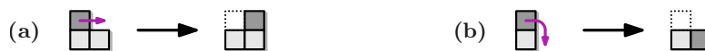
■ Figure 1 Moves admitted by the sliding cube model: (a) slide, (b) convex transition.
