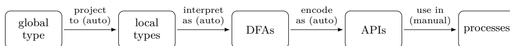
■ Figure 4 Workflow of API generation (the first three arrows are performed automatically by the tool; the last arrow is performed manually by the programmer).
