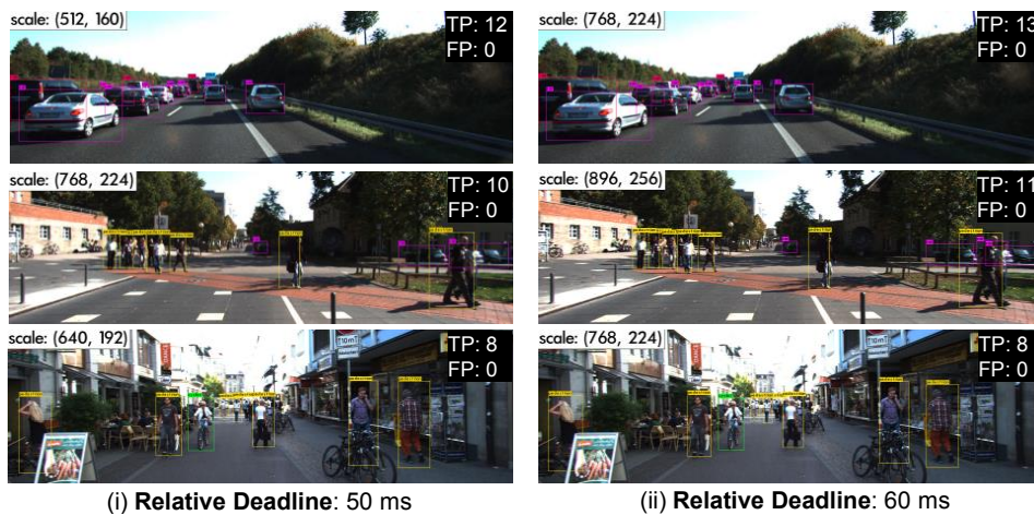
■ Figure 11 Sample object detection results with the image scales used in detection (TP: True Positive, FP: False Positive).
