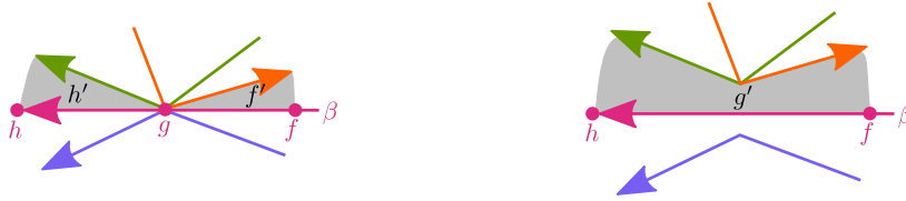
■ Figure 7 Before (left) and after (right) a merge phase. The (shaded) face g' is obtained by merging faces h' and f' .
