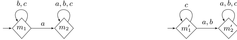
■ Figure 1 Memory skeletons \mathcal{M} (left) and \mathcal{M}' (right) for two-target reachability games. In figures, diamonds (resp. circles, squares) represent memory or automaton states (resp. arena vertices controlled by \mathcal{P}_1 , arena vertices controlled by \mathcal{P}_2 ).
