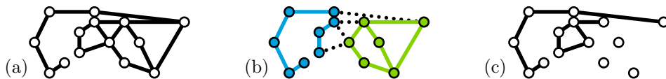
■ Figure 1 (a) A planar graph G . (b) A set \beta \subset V and \gamma \subset V . We show G[\beta] and G[\gamma] . The set G[\beta] \cup G[\gamma] contains no black edges. (c) We show G \setminus G[\beta \cup \gamma] .
