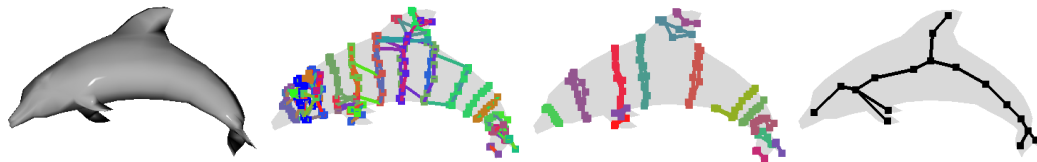
■ Figure 2 Visualisation of the three phases of the LSS algorithm. From left to right: A shaded render of the input, a number of computed minimal separators, a non-overlapping subset of the separators, and the resulting skeleton after extraction.
