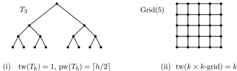
■ **Figure 15** (i) The complete binary tree  $T_h$  of height  $h$  has pathwidth  $\lceil h/2 \rceil$ , cf. [10, Theorem 67]. (ii) The  $k \times k$  grid graph is known to have pathwidth and treewidth both equal to  $k$ .
