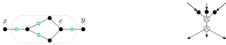
(a) Gadget simulating an implication arc from x to y using booster edges (marked with green diamonds).
