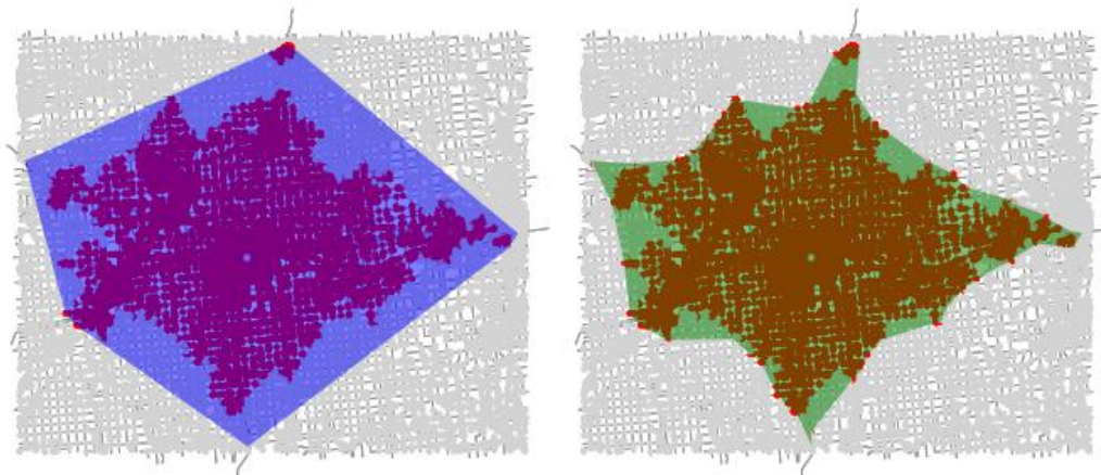
■ Figure 1 An example of the difference between convex hulls and alpha shapes on road network data. The street network nodes in red are within 30 minutes of the Carle Hospital in Urbana, IL while the grey nodes are not. The convex hull around the red nodes is on the left and the alpha shape (with \alpha = 2^{-13} using Albers Equal Area Conic projection) is given on the right.
