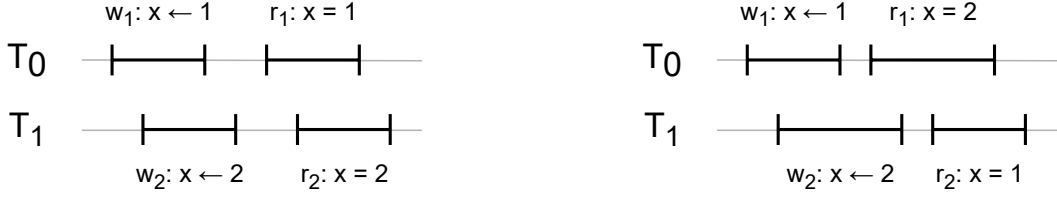
(a) A schedule allowed by the weak, read-from and no-inversion definitions but not by our regular register model.
