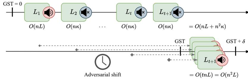
■ **Figure 2** The *adversarial shift* attack on  $t + 1$  leaders. The first line shows how leaders are optimistically ordered in time by the protocol to avoid redundant broadcasts (the blue speaker circle represents an *avoided* redundant broadcast). The second line shows how leaders can slow down before GST and overlap at GST, making redundant broadcasts (seem) unavoidable.
