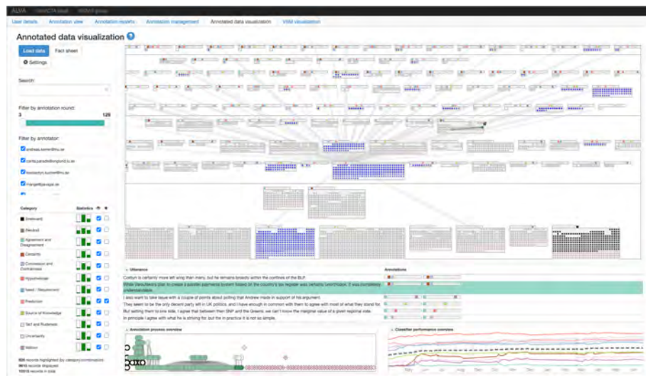
■ Figure 11 One of the interactive visual interfaces in ALVA represents the current contents of the annotated dataset with a focus on combinations of labels, the data about the annotated process, and the data about the performance of the respective machine learning classifier trained over time with additional labeled data according to the active learning approach.
