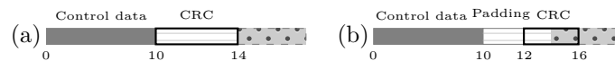
■ Figure 1 Mis-interpretation of a MAC ACK frame by an Atheros receiver: (a) Layout of the incoming ACK frame and (b) The type-incompatible layout computed by the receiver
