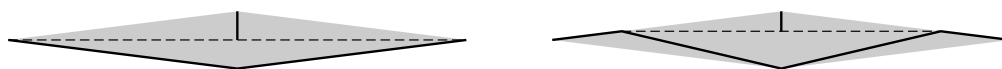
■ Figure 7 Two barriers for a rhombus with shorter diagonal of length 2 and with sides of equal length a \geq 4 . Left: The barrier found by Shermer's procedure. Right: The barrier found by Provan et al. [23]. The height from the top vertex to the dashed line in the right barrier is b \leq 1 .
