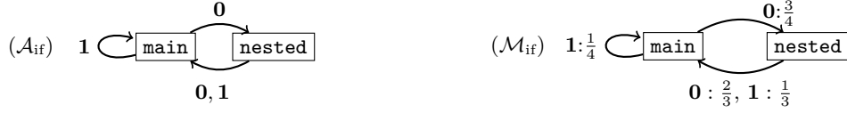
■ Figure 11 On the left, the automaton \mathcal{A}_{\text{if}} . On the right, the Markovian automaton \mathcal{M}_{\text{if}} of transition probabilities \mathbb{P}(1 \mid \text{main}) = \frac{1}{4} , \mathbb{P}(0 \mid \text{main}) = \frac{3}{4} , \mathbb{P}(0 \mid \text{nested}) = \frac{2}{3} and \mathbb{P}(1 \mid \text{nested}) = \frac{1}{3} .
