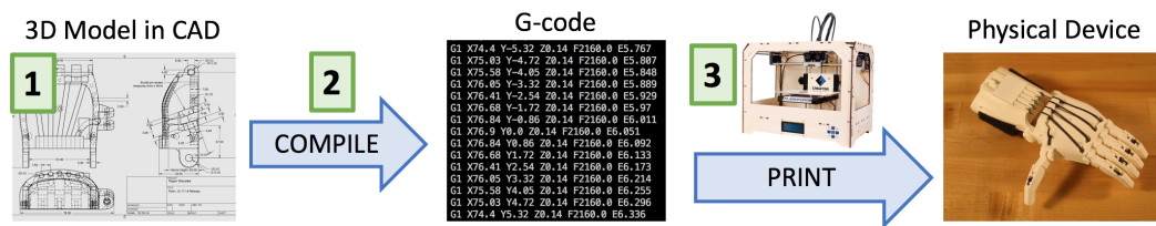
■ Figure 1 The 3D Printing Development Cycle. To 3D print a device: (1) An engineer first designs a 3D model using standard CAD tools (e.g., SolidWorks [28]). (2) This model is compiled into a sequence of low-level G-code commands that corresponds to basic actions the printer can take (move the print head, start/stop extrusion, lower the build plate, etc.). (3) The printer directly executes the G-code , producing a physical object.
