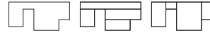
■ Figure 3 A shape to be formed (left) and the possible rectangle decompositions thereof (middle, right).
